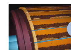
P7 Burning mark of commutator segment(P7)
