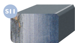
S11 Copper precipitates (S11)
